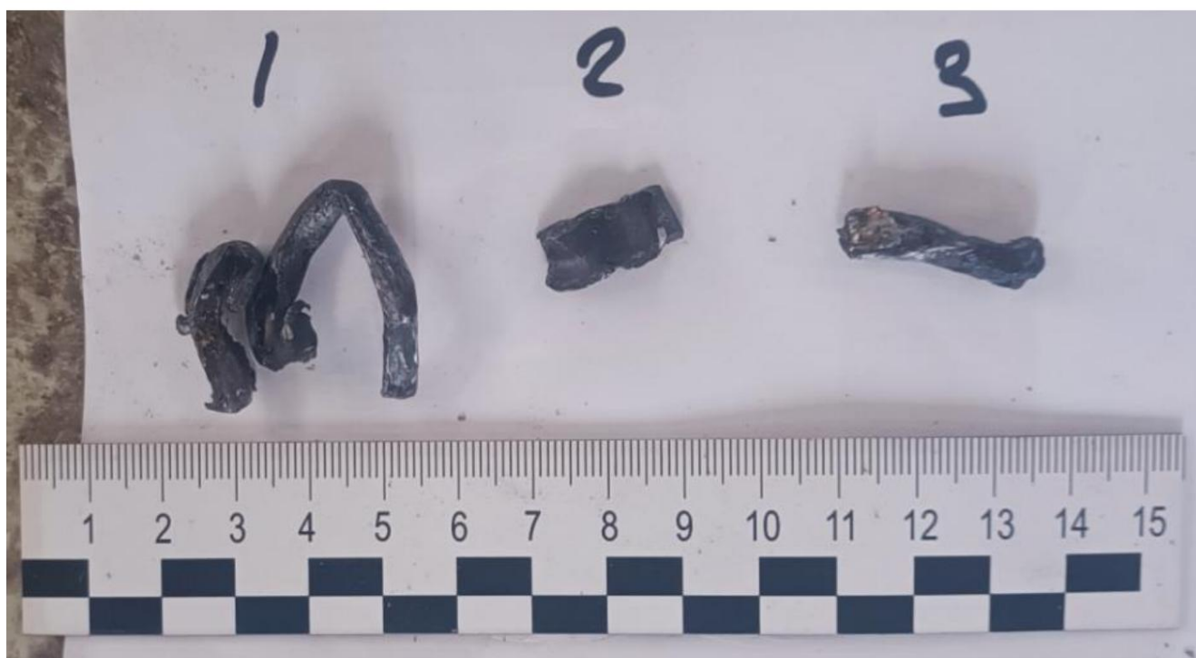
Fig. 22. Part of the foreign metal objects removed from hydraulic system compartment No. 3 and the stabilizer control mechanism
