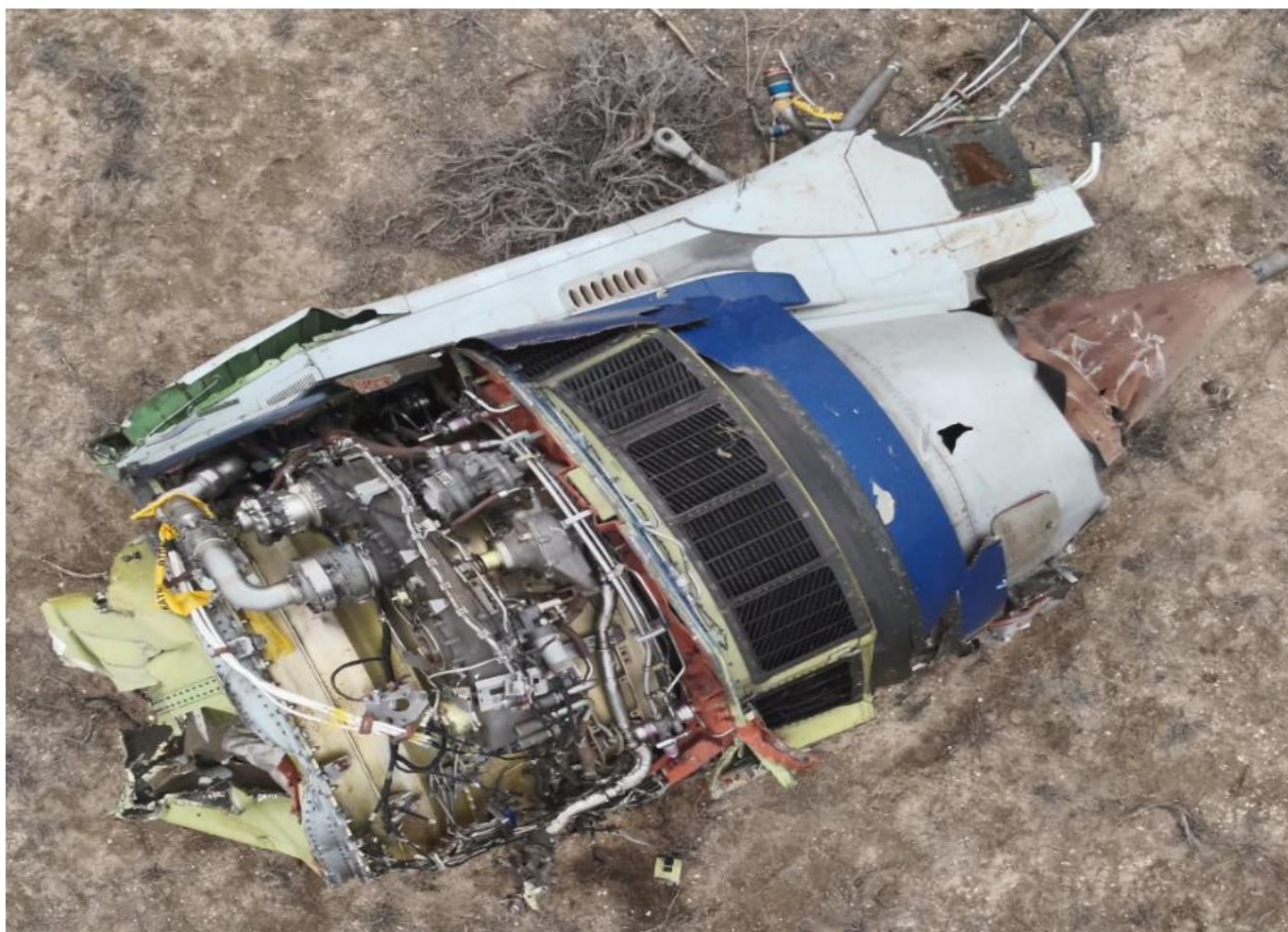
Fig. 8. Left engine with part of the pylon
