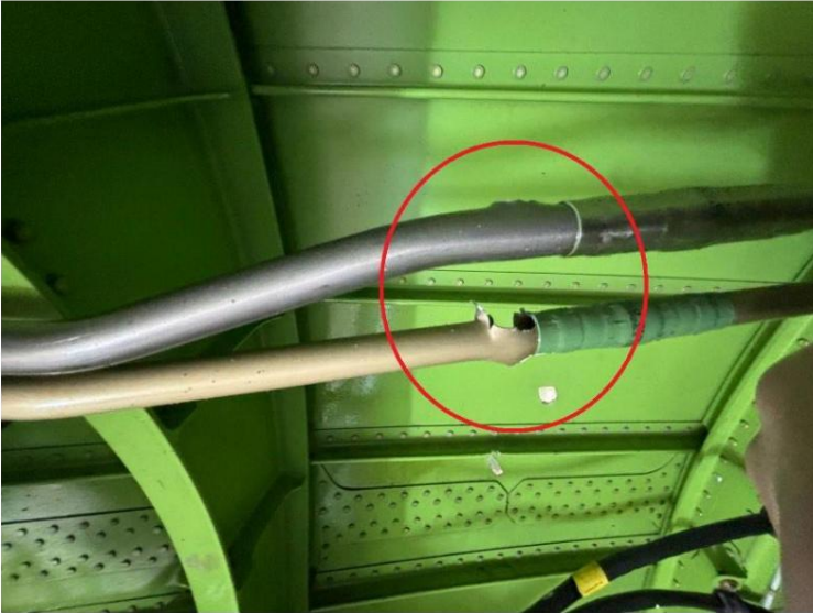
Fig. 13. Hydraulic system 1 – Damaged tube
