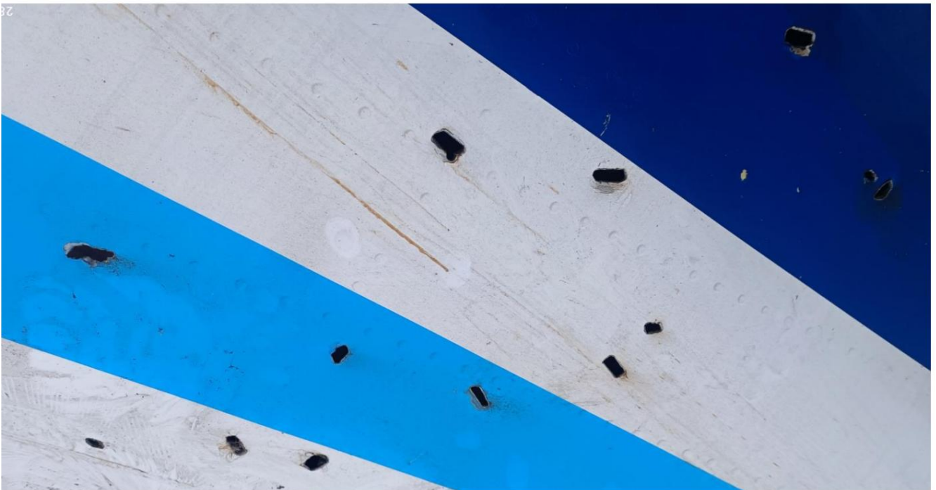
Fig. 11. Damage to the left side of the tail section
