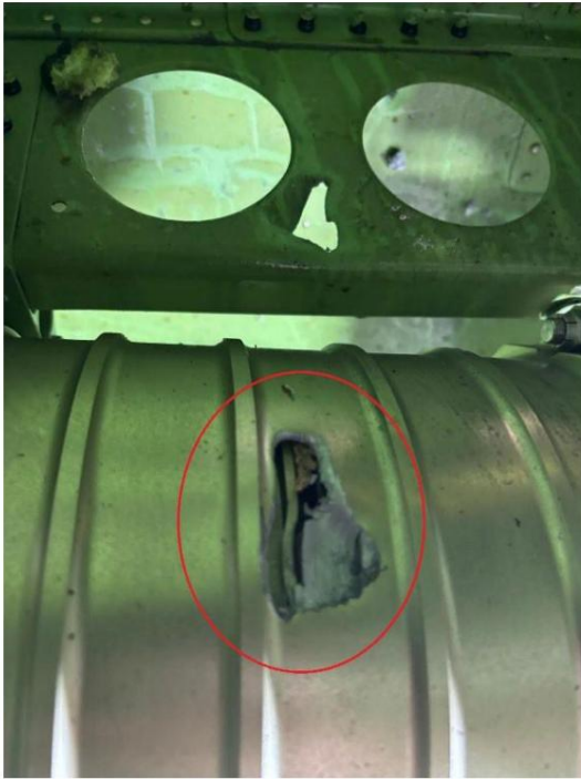
Fig. 18. Hydraulic system 3 – damaged tank
