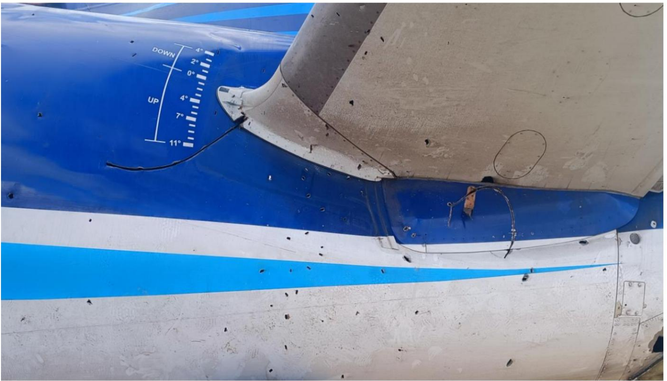
Fig. 10. Damage to the left side of the tail section
