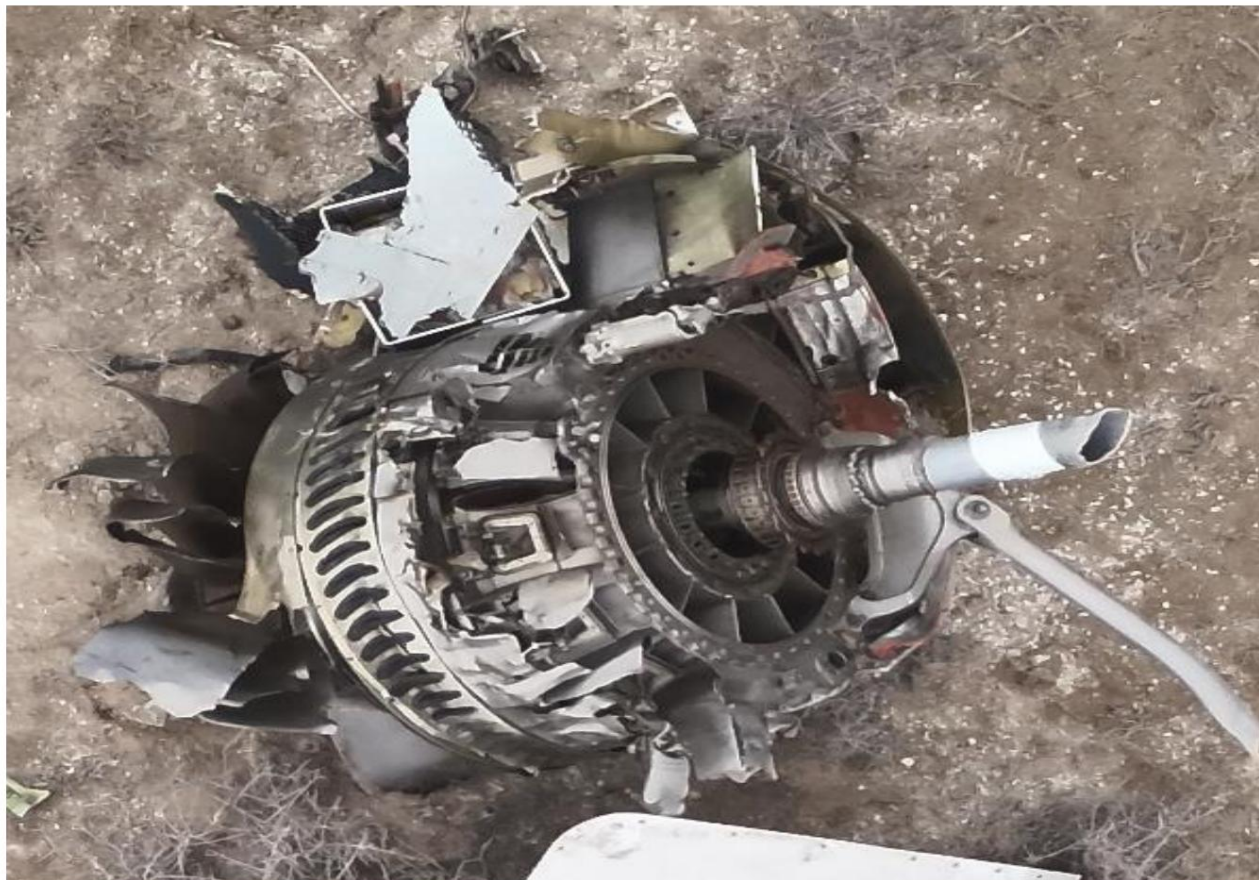
Fig. 7. Front part of the right engine
