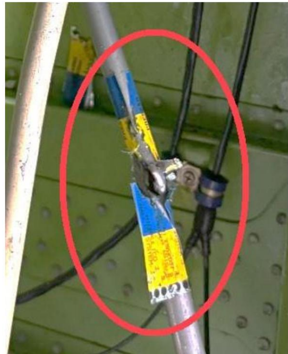
Fig. 16. Hydraulic system 3 – detailed view of the damaged tube
