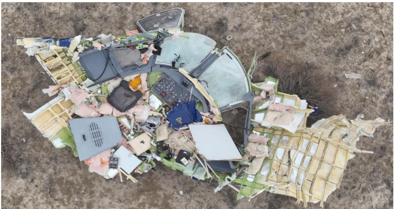
Fig. 6. Cabin canopy and upper panel
