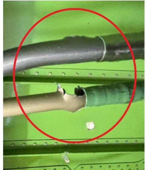
Fig. 14. Hydraulic system 1 – Damaged tube - detailed view
