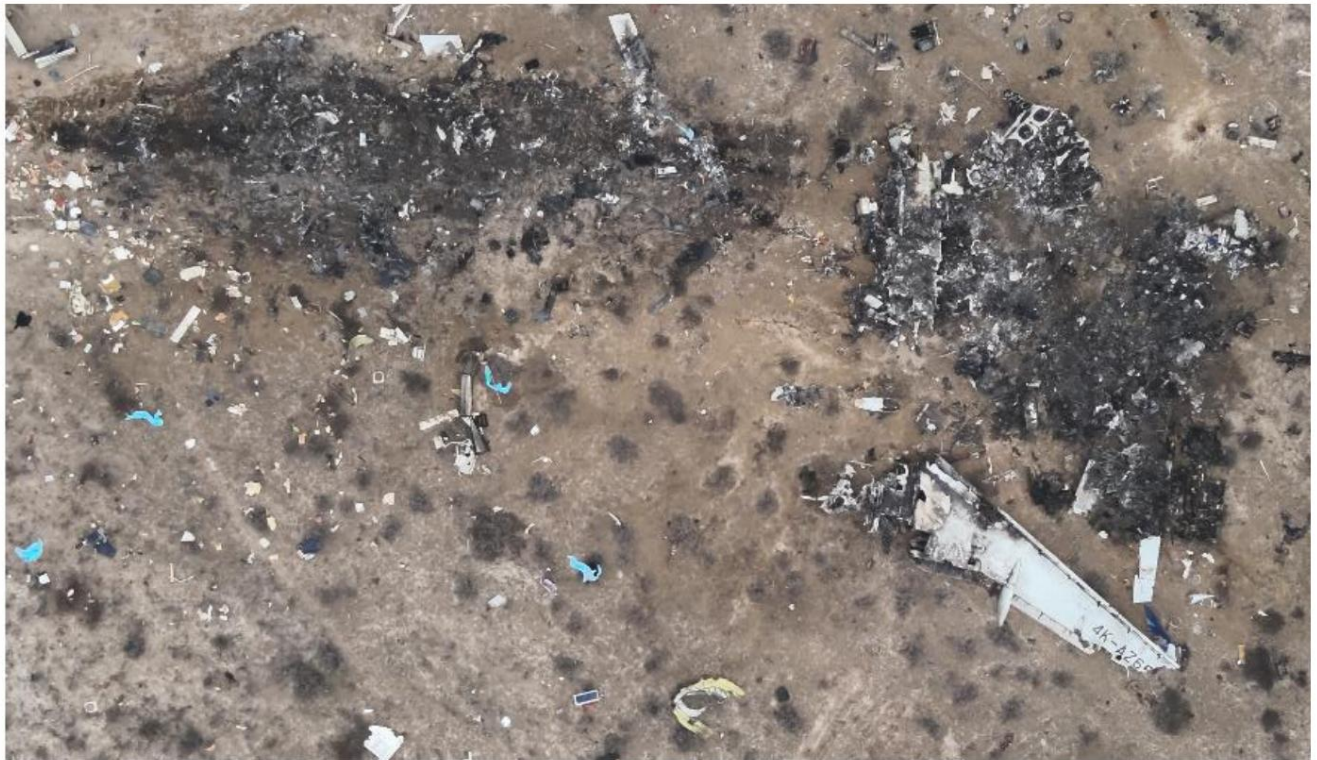
Fig. 5. The main source of the fire (right wing, nose and center sections of the fuselage, center section and left wing)
